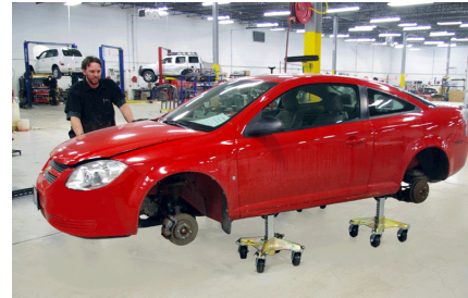
RapidGlide units roll very easily – when moving on a hill or incline always have assistance
